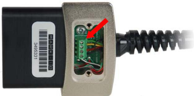
2. Feed the four leads through the supplied strain relief (pictured above) and into the body of the adapter.
