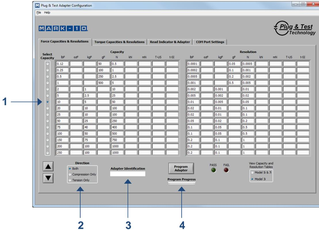
Use the **Force Capacities & Resolutions** and **Torque Capacities & Resolutions** screens to program the capacity appropriate for the sensor. The number of available units of measurement and displayed resolution depend on the indicator being used. Refer to Section 5 for detailed information.
