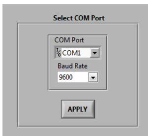
Use this screen to configure the PC's COM port to which the indicator is connected.
